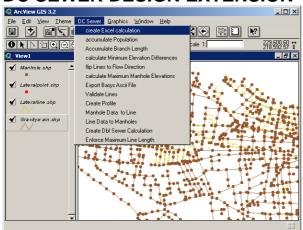
**DC SEWER DESIGN EXTENSION** is the free ArcView 3.x solution for analyzing and displaying simple wastewater networks developed by DORSCH CONSULT.
